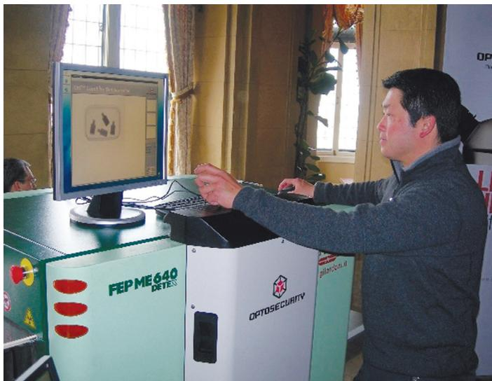
Optosecurity has developed an add-on X-ray screening upgrade that can quickly scan liquids for explosive traces.
